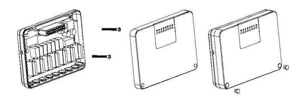
Screw for mounting thermostat to wall
