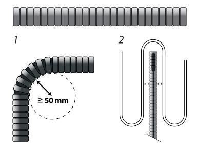
The bending radius of the conduit must be min 50 mm.
